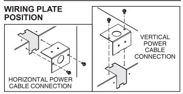
Wiring plate mounts to side or top of housing.
