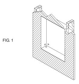
NOTE: IN THE VERTICAL POSITION THE HEATER CAN BE MOUNTED ONLY FOR TOP DISCHARGE. FIELD WIRING MUST ENTER THE BOTTOM ON THE LEFT SIDE OF THE HEATER.
